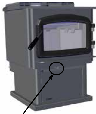
Primary Air Damper Left - Open Right - Closed
