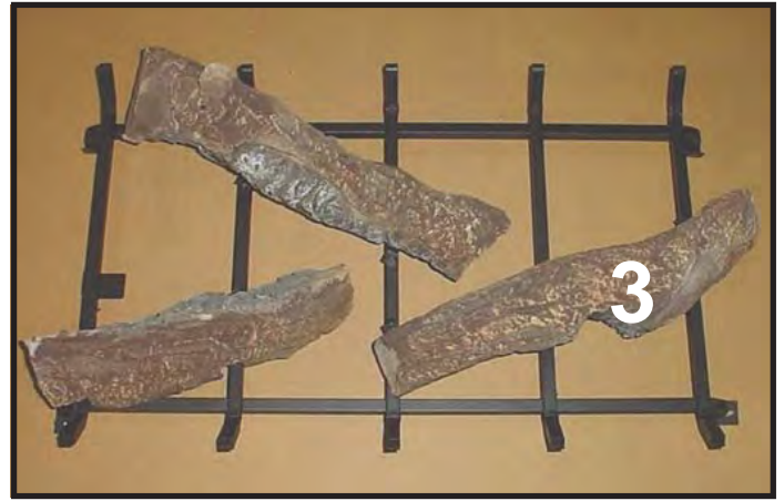
LOG #3 (SRV2068-702): Position log #3 across the third, fourth and fifth grate bars and push towards the rear against the grate tabs on bars three and five.
