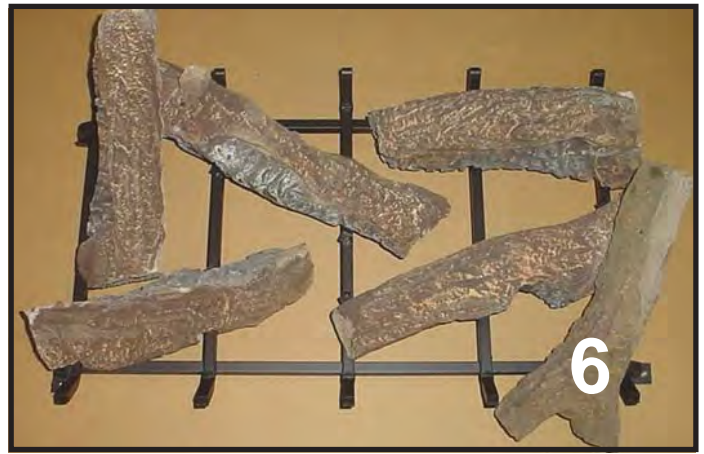
LOG #6 (SRV582-705): Position log #6 on top of the groove in log #3 with the forked end resting on the grate assembly as shown.
