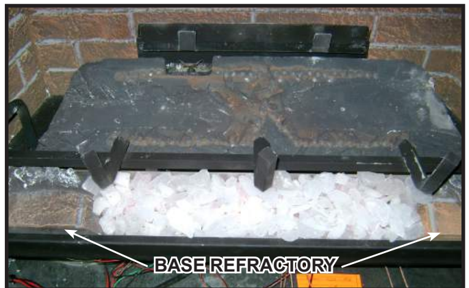
Figure 11.6 Install Base Refractory
