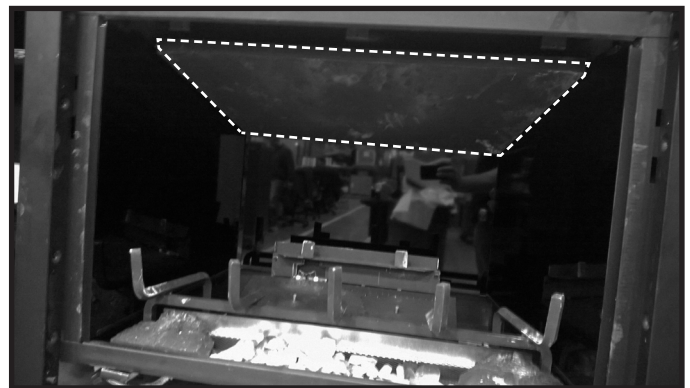
Figure 11.5 Install Top Refractory Panel
