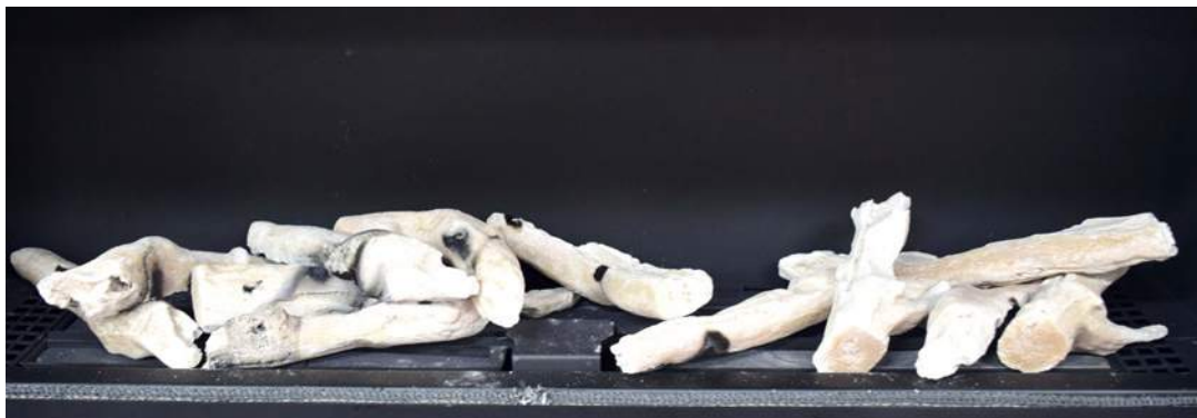
Incorrect Media Installation
