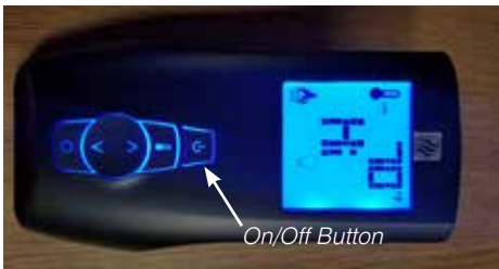
Diagram 1 Remote shown in Manual Mode on Hi
