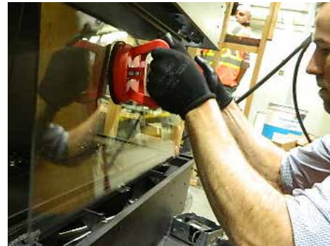
Handle front panel with supplied vacuum clamps
