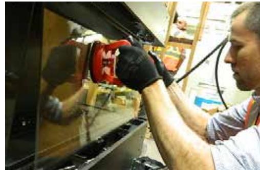
Handle front panel with supplied vacuum clamps
