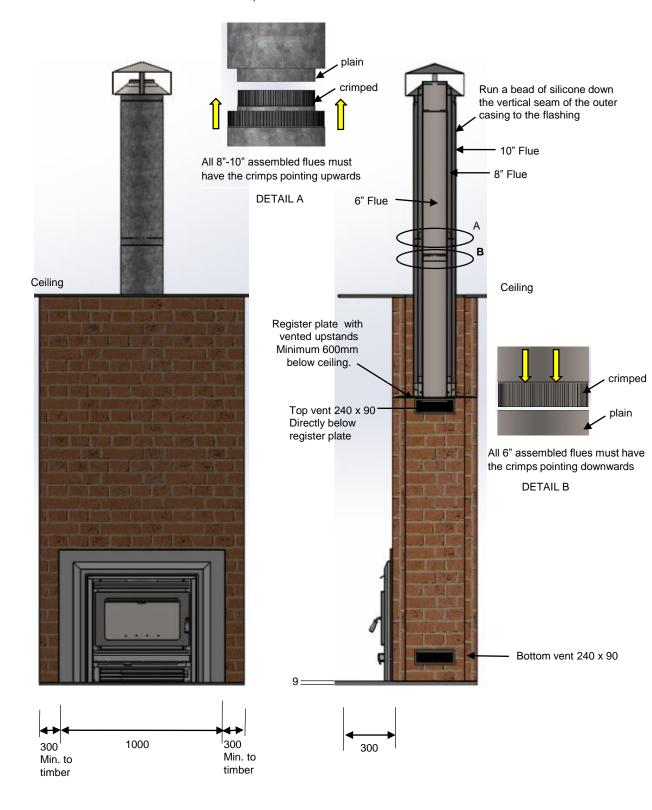
Alternate finish to full masonry chimney
