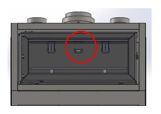
1. REMOVE MIDDLE AIR TUBE BY PUSHING UP AND REMOVING FROM FRONT AND REAR BRACKETS.
