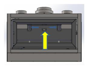
2. PLACE ALL 4 BAFFLE PLATES ABOVE AIR TUBES BOTH SIDES CLOSEST TO THE FIRE BOX WALL AS SHOWN ( 2 LEFT AND 2 RIGHT)
