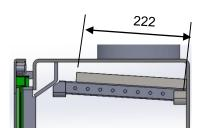
3. PLACE BAFFLE PLATES AS FAR BACK AS POSSIBLE, 222 MM FROM FRONT TO BACK.
