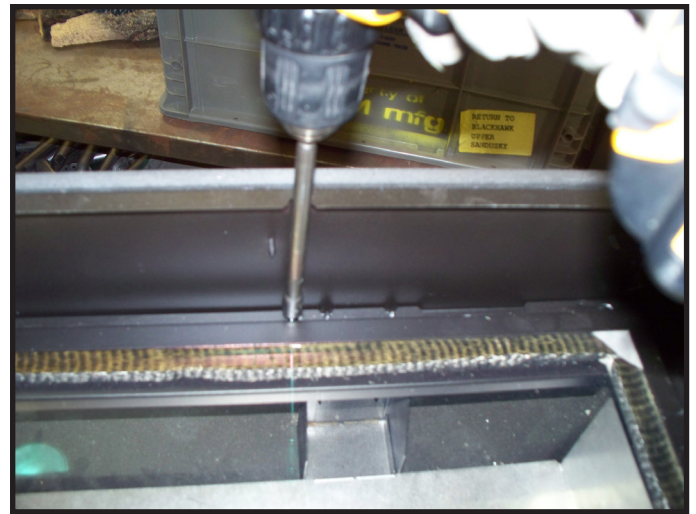
Figure 9.4. Gas and Electrical Access - Remove Glass Window
