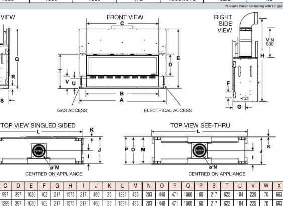
Dimensions above are in millimetres and for reference only. We recommend measuring individual units at installation. Refer to installation manual for detailed specification on installing this product. Heat & Glo reserves the right to update units periodically. The flame appearance may vary based on the type of fuel burned and the venting configuration used. Photos in this brochure may vary in colour and dimension (size) from the actual product.
